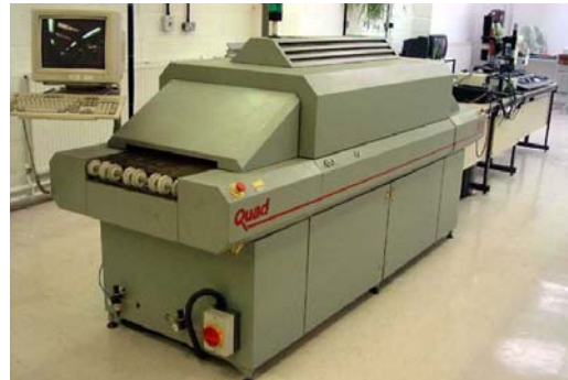
Lot No 207 Quad Zone Convection Re-Flow System with Extraction System, Monitor & Printer
