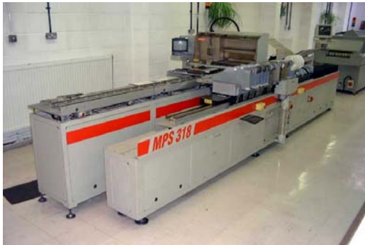
Lot No 206 Dynapert MPS 318 Surface Mount Placement Machine (4500 placements per hour)
